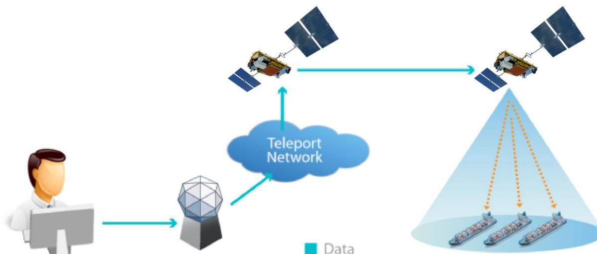
**Figure 2 – Basic concept of the Iridium SafetyCast service**
