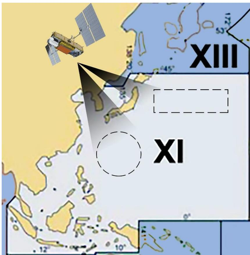
**Figure 5b – Examples of message addressing to circular and rectangular areas**
