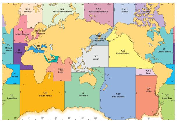
Figure 2: NAVAREAs for coordinating and promulgating navigational warnings under the World-Wide Navigational Warning Service within the GMDSS
