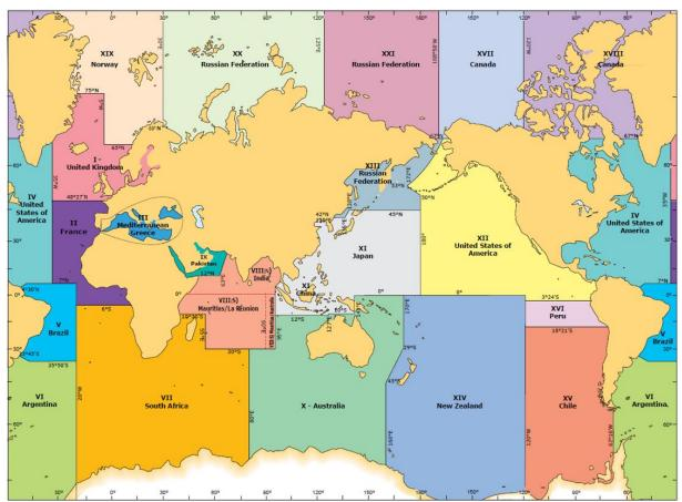
Figure 3: METAREAs for coordinating and promulgating meteorological warnings and forecasts under the Worldwide Met-Ocean Information and Warning Service within the GMDSS
